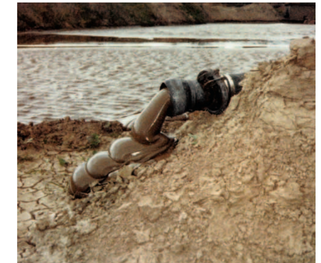
Abrasive sludges with a high concentration of solid mater can be transported without problem.
